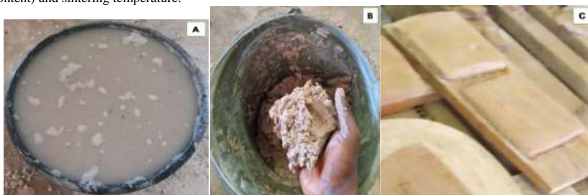
Figure 1: (A) Raw materials soaked in water. (B) Slip for tile making, (C) Produced ceramic tiles
